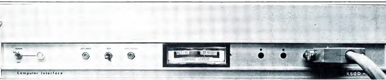
The power supply, unique logic circuitry and relays of the Automate-64 system fit in a 2-inch-high standard rack.
